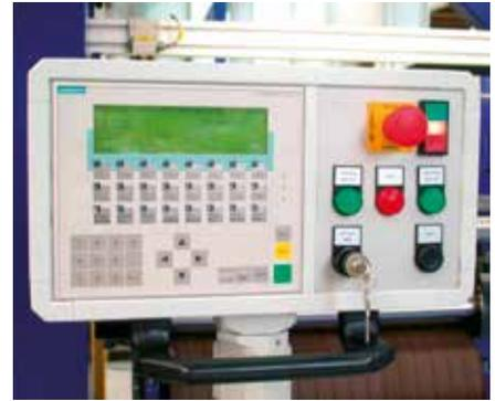
From the Siemens operator panel, each step in the TWINMASTER process is monitored and controlled. Weil Engineering uses ProTool software to custom configure the HMI on the machine.
