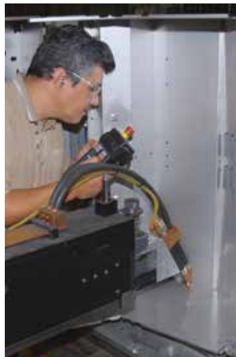
Contour-Arc CNC spot welding system, developed to produce various sizes and styles of end products with minimal changeover time.
